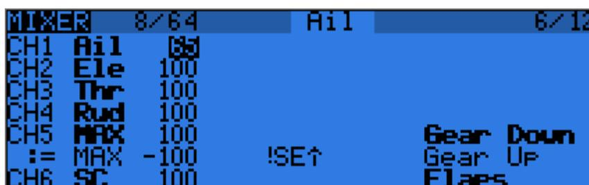
The various channels are outputs, for example CH1 being the servo plug #1 on your receiver (with the default protocol settings). A channel without a mixer line will just centre a servo that would be connected to it. Each mixer line connects one input to the channel it's on. Inputs can be:
